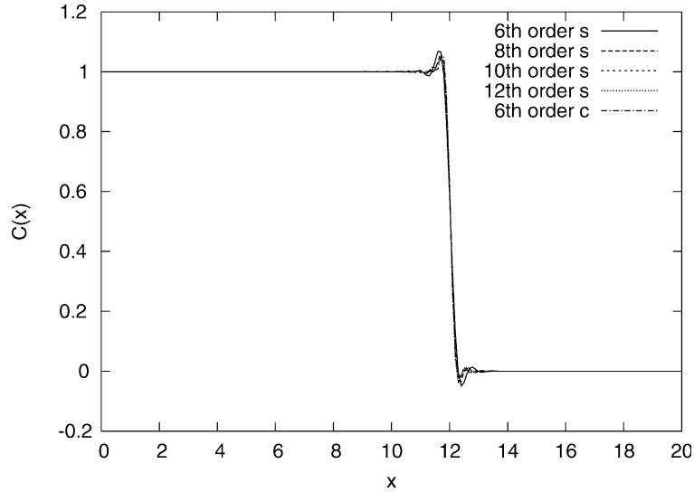
Fig. 5. Advection of a passive scalar with different orders of the spatial discretization, (s) denotes a staggered formulation and (c) a collocated formulation.
